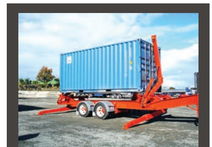
The TRT-designed 3-crane Sideloader will now be produced by HAMMAR New Zealand.
